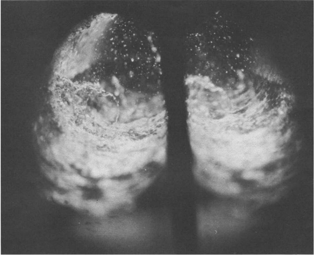
FIG. 4. Stereo and semi-axial photography of annular two phase flow (Whalley et al. [23]).
